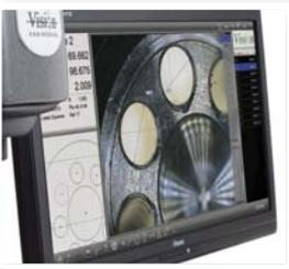
'Next generation' measurement software coupled with a high resolution video camera allows Falcon to measure a wide variety of simple and complex features, quickly and simply.
