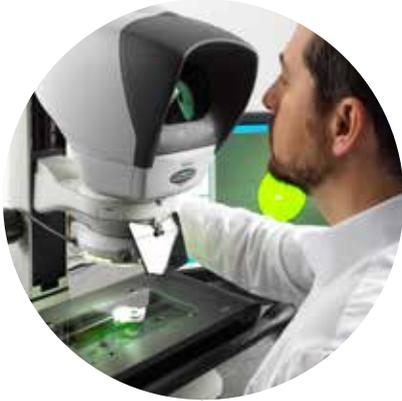
between surfaces is viewed so both sides of the surface can be seen. In direct down views a vertical surface can't be seen so the view of the intersection is not as clear. Lynx EVO and EVO Cam II both feature a 360° viewer.
